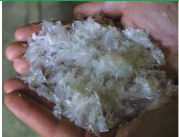
Washed PET flakes from used beverage bottles at the Eko-Kom facility in the Czech Republic. These flakes will be sold and reused in other industrial applications.
